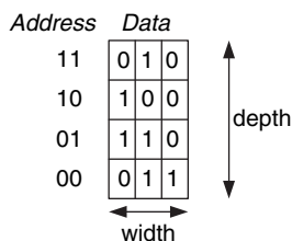
Figure 5.40 4 × 3 memory array: (a) symbol, (b) function
