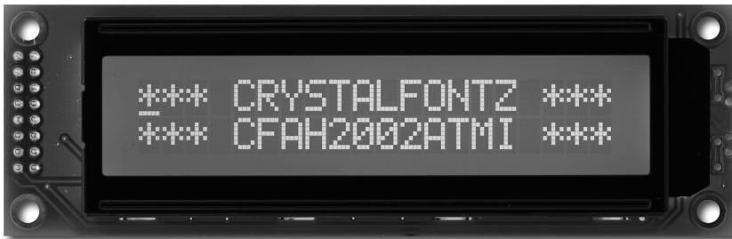
Figure e9.24 Crystalfontz CFAH2002A-TMI 20 \times 2 character LCD (© 2012 Crystalfontz America; reprinted with permission.)
